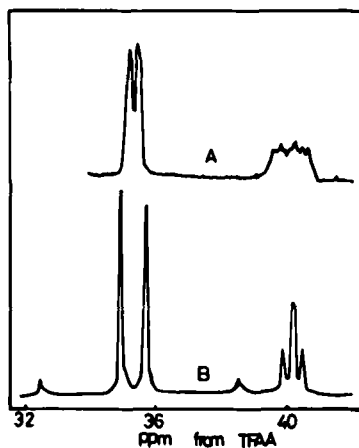
Fig. 13. Fluorine NMR spectra of IB-CTFE copolymer polymerized at 0°C. (A) 56 Mc, (B) 94 Mc. Measurement was carried out in C_2Cl_4 at 100°C.
